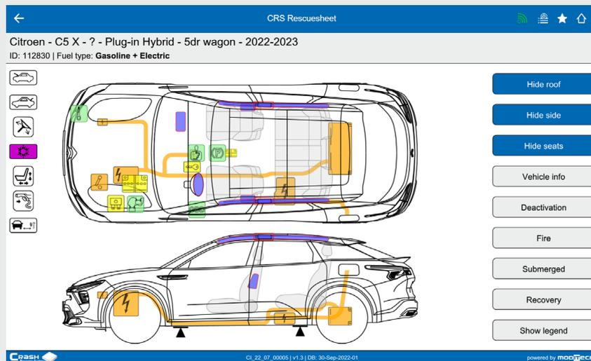
The interactive top and side views show all relevant components (shown in green) such as the battery, tow bar, (electric) parking brake and locations such as the fuse box in one overview. In the case of a hybrid or electric vehicle, the roadside assistance provider is immediately informed of deactivation procedures after selection of the vehicle. Additional information is easily accessible by clicking on the various components in the vehicle image.
