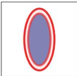
Dangerzone driver and passenger airbag. Driver and passenger airbags outlined in **red indicate** dual stage airbags, whereby one stage may remain active after activation of the airbag. It also indicates a mechanical driver airbag which can be activated using mechanical force.
