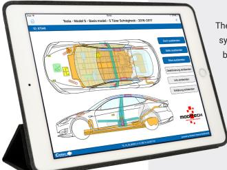
The interactive top and side view of the vehicle shows all safety systems present and other relevant components (such as the battery, fuel tank, etc.) at a glance.
