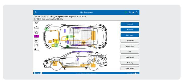
The interactive top and side views show all relevant components (shown in green) such as the battery, tow bar, (electric) parking brake and locations such as the fuse box in one overview. In the case of a hybrid or electric vehicle, the roadside assistance provider is immediately informed of deactivation procedures after selection of the vehicle. Additional information is easily accessible by clicking on the various components in the vehicle image.
