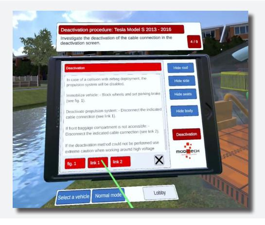
The next Step is now above the tablet: 5/9 "Cut the emergency disconnect cable on the front right under the bonnet."
