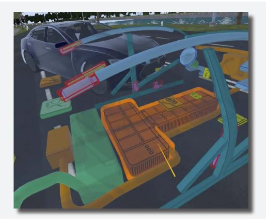
This completes the step. The tablet now reads: "The thermal imaging camera indicates that the battery has not warmed up (yet). No liquid leakage or smoke is visible."
