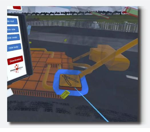
The next Step is now above the tablet: 8/8 "Cut the Emergency disconnect cable in the C-pillar by viewing Figure 1"
