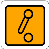
High voltage device that disconnects high voltage
