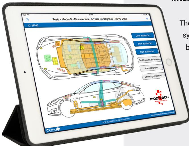
The interactive top and side view of the vehicle shows all safety systems present and other relevant components (such as the battery, fuel tank, etc.) at a glance.
