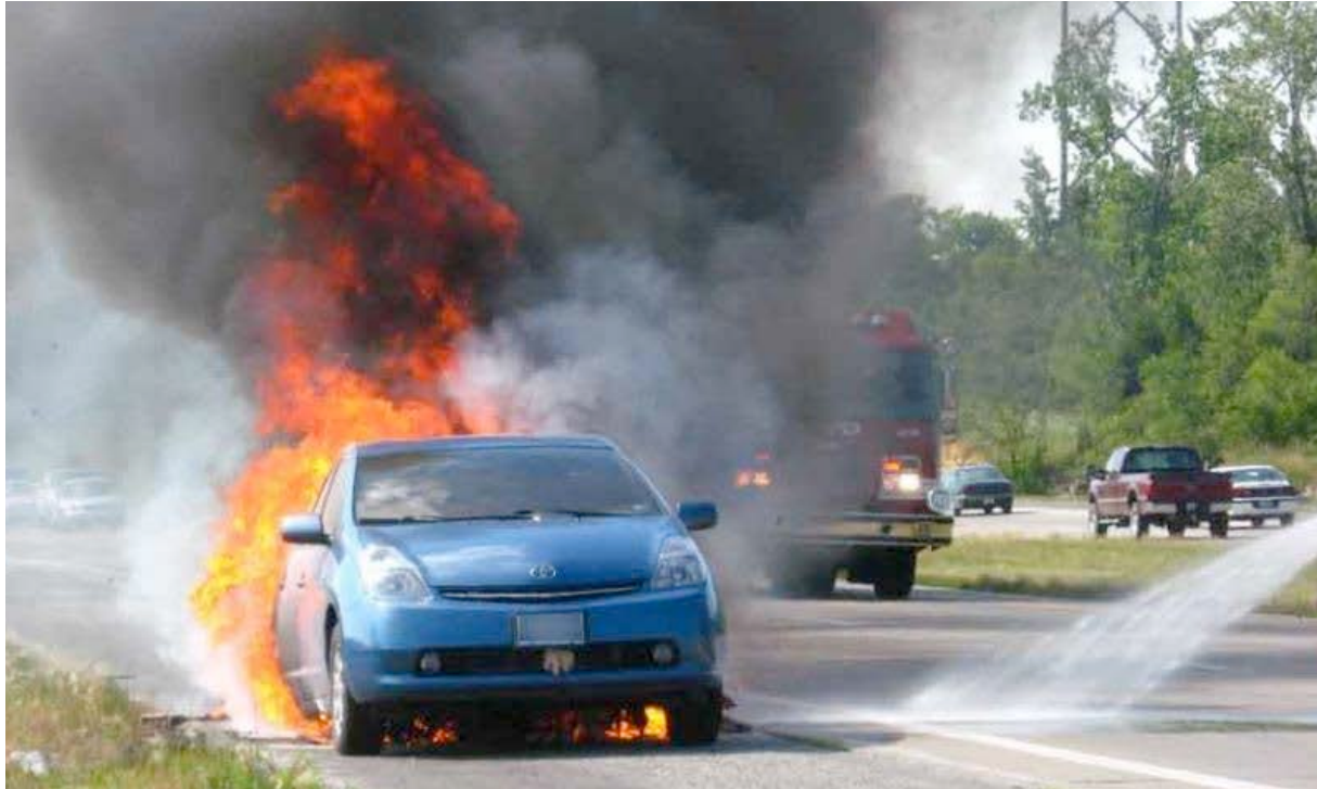
Figure 32: Vehicle fire involving a Toyota Prius Hybrid vehicle. The vehicle is a total loss and cannot be repaired. It does not make sense to take a risk!
