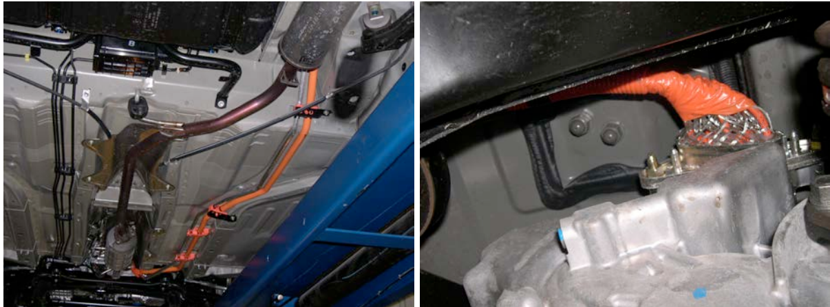
Figure 14: High voltage power cables under the floor pan of Hybrid vehicles (Honda Civic IMA, Lexus RX 400h). In the right photo the wire braid that is used for insulation monitoring is visible.
