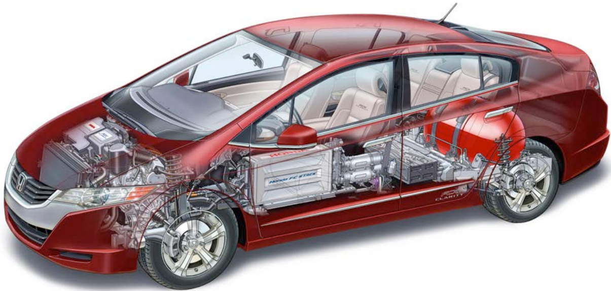
Figure 17: Honda FCX Clarity test vehicle. In this vehicle the hydrogen is stored under pressure (345 bar) and feed a fuel cell. The fuel cell creates electricity to power an electric motor. A high voltage battery is also present (courtesy of Honda).
