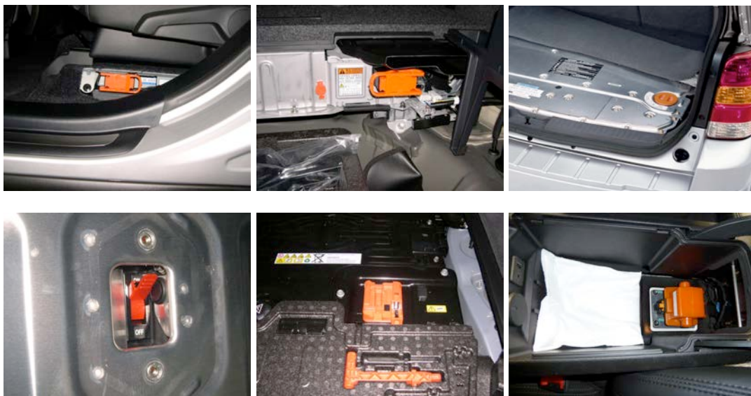
Figure 15: Examples for different service disconnect switches.
