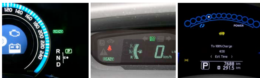
Figure 26: Examples for 'ready'-indicators on different hybrid- and electric vehicles.
