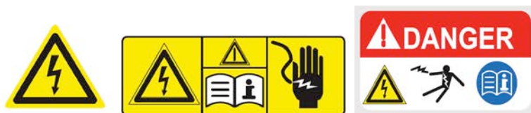
Figure 13: Identification label for high voltage components
