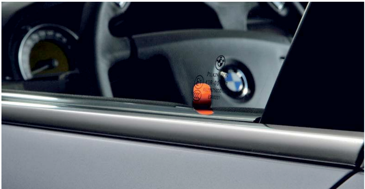
Figure 24: Gas warning system of BMWs Hydrogen7 vehicle. The LEDs of the gas warning system are integrated into the door pins and start flashing if hydrogen is detected (courtesy of BMW).
