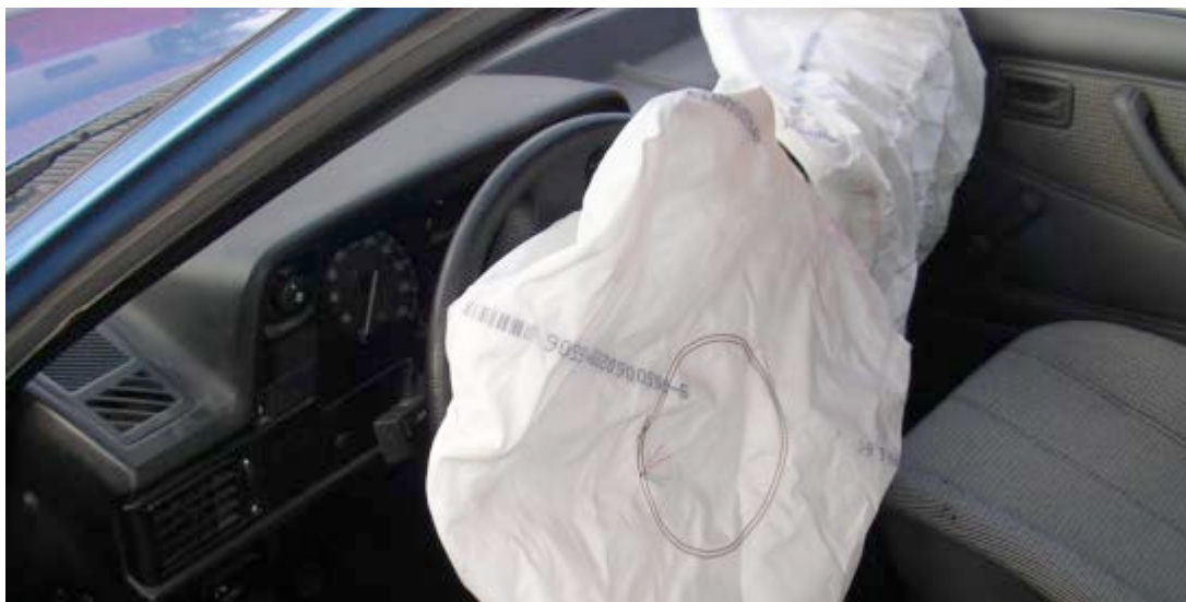
Figure 34: Retrofitted deployed driver and passenger airbags
