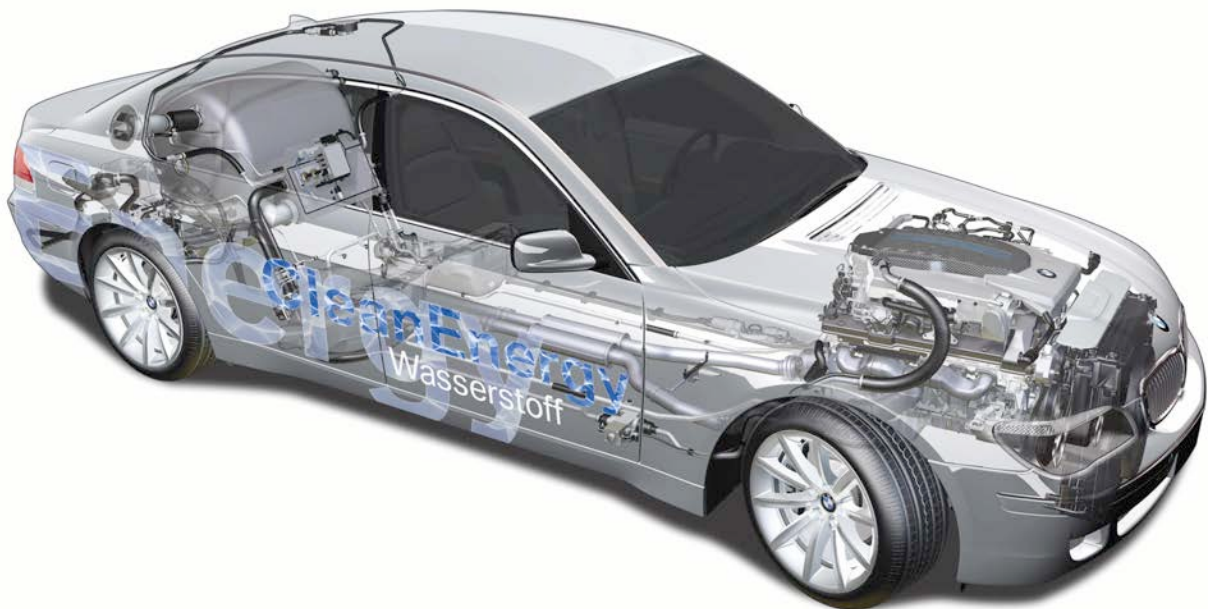
Figure 16: BMW Hydrogen7 test vehicle with hydrogen propulsion. On this vehicle hydrogen will be stored liquefied at -253 °C and burned in an internal combustion engine (courtesy of: BMW).
