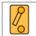
Service/Emergency disconnect switch
