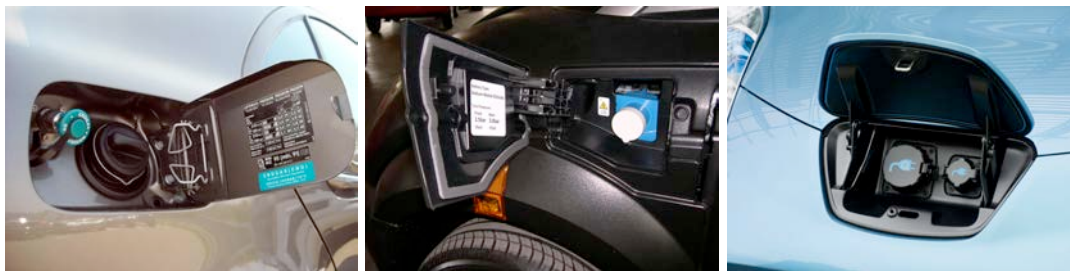
Figure 22: Different filler caps. a. bivalent Gasoline/CNG-vehicle, b. Electric vehicle, charge connector in the front fender, c. Electric vehicle, two charge connectors on the front of the vehicle.
